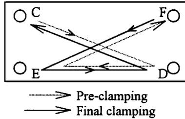
Figure 55. Clamping Order for Four-point Clamping Module
