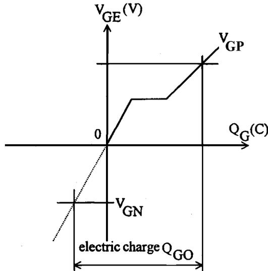
Figure 27. Driving Voltage and Gate Electric Charge
