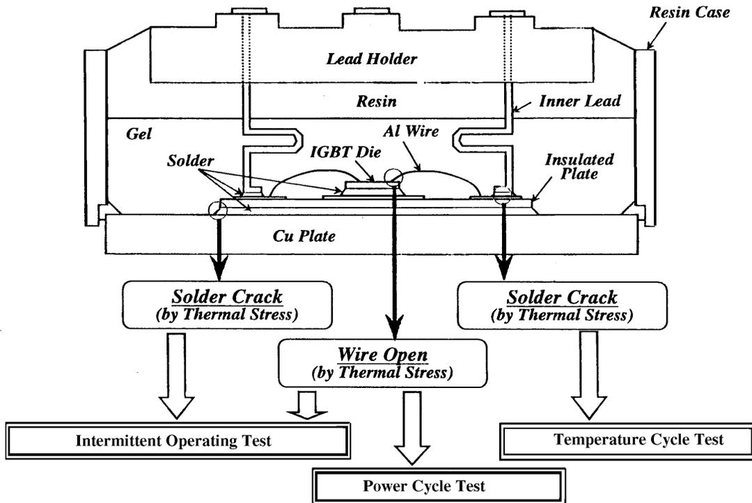
Figure 59. Possible Failure Mechanisms for an IGBT Module
