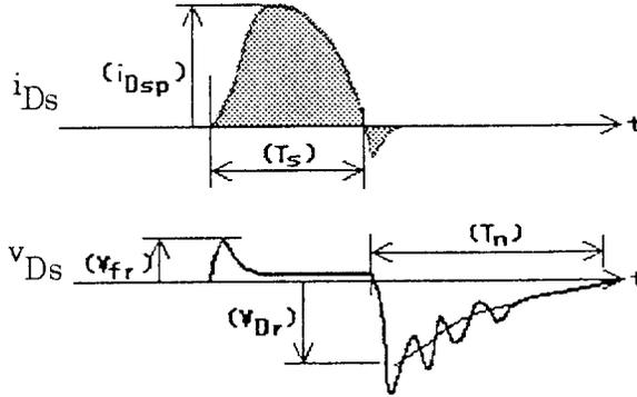
**Figure 24. Snubber Diode Current and Voltage Waveforms**
