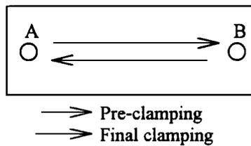
Figure 54. Clamping Order for Two-point Clamping Module
