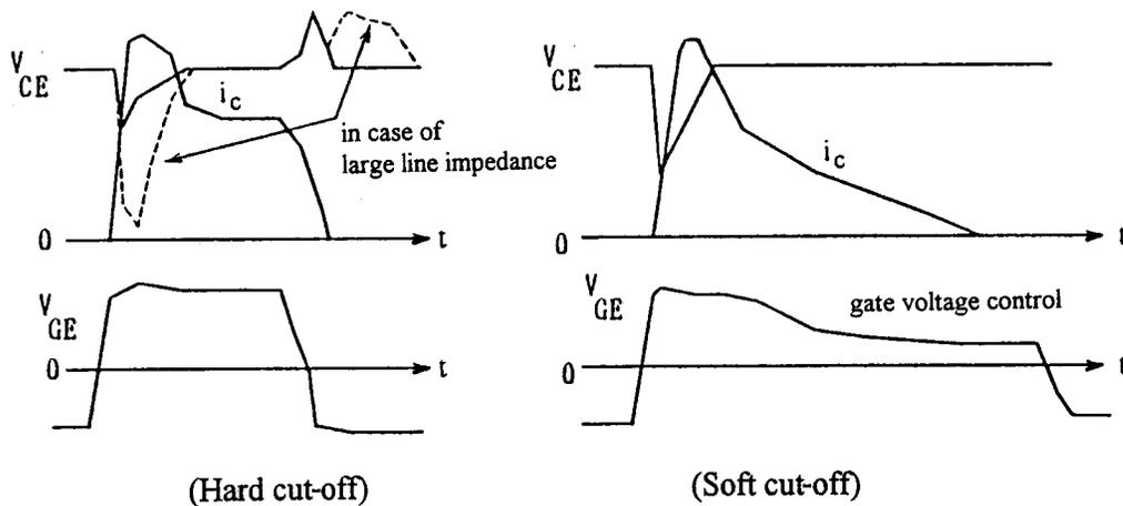
Figure 50. Short-circuit Protection Waveforms
