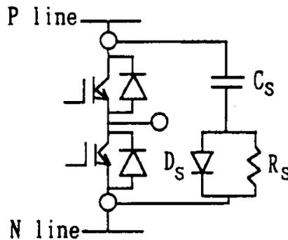
Figure 18. Snubber Circuit between P and N
