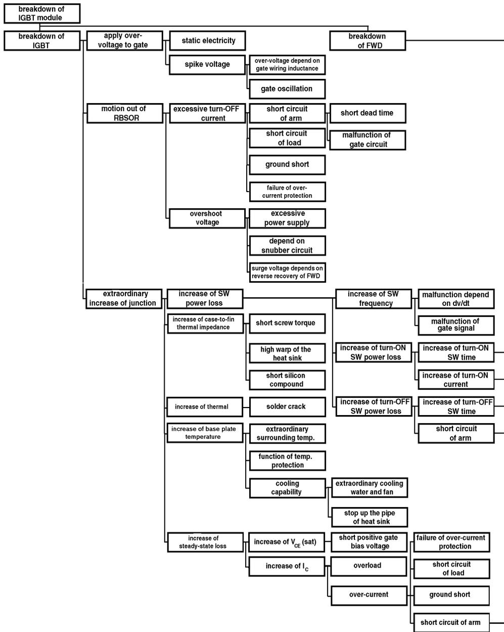
Figure 60. Electrical Failure Analysis
