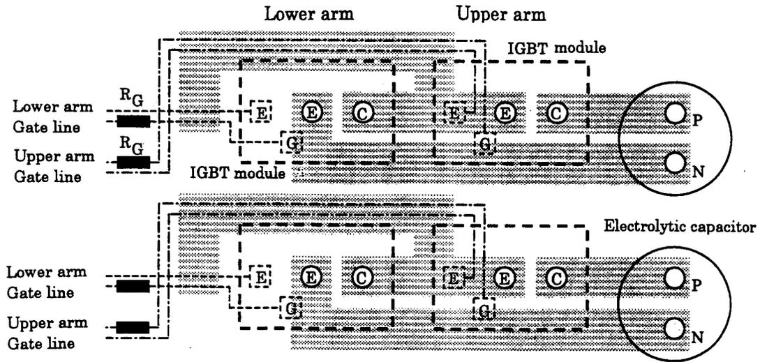
Figure 32. Example of Parallel Connection Wiring
