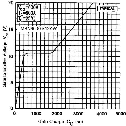
Figure 8. Gate Charge Characteristics
