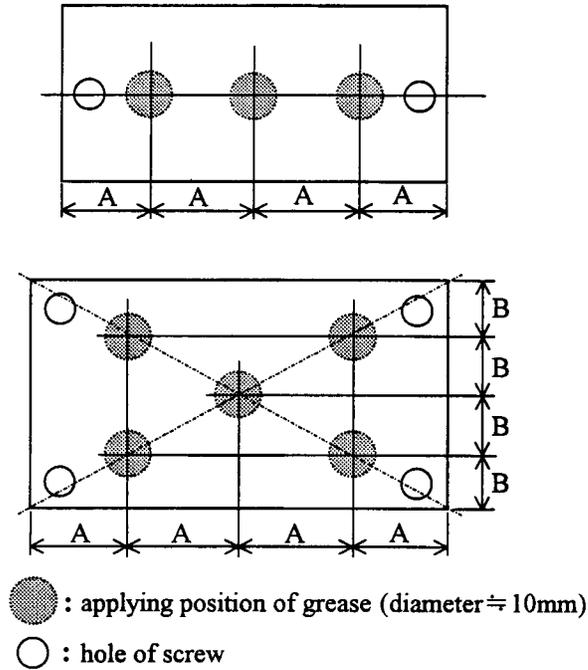
Figure 53. Grease Positions
