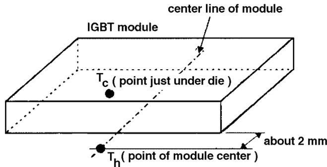
Figure 36. Definition of  $T_c$  and  $T_h$  Measurement Points
