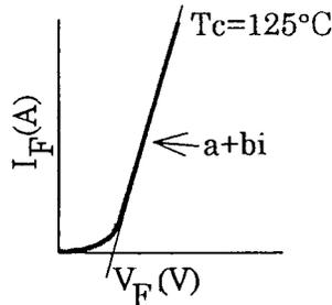
Figure 35. Forward Voltage Characteristics of Free-Wheeling Diode
