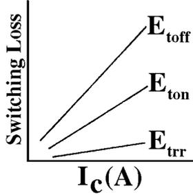
Figure 34. Switching Loss vs. Collector Current
