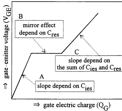
**Figure 26. Example of Gate Electric Charge Characteristics**
