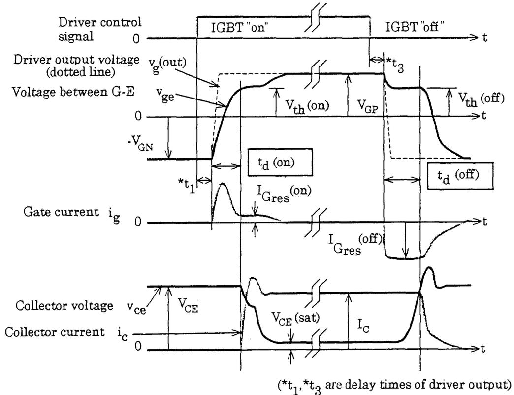
Figure 43. Inductive Load Turn-ON and Turn-OFF Switching Waveforms
