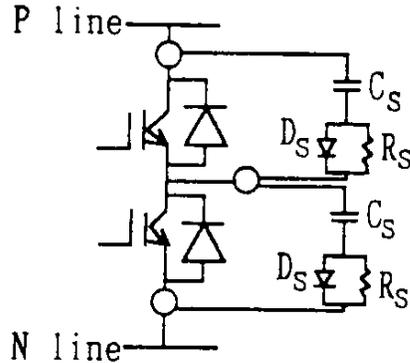
Figure 20. Pair of Snubber Circuits between Arms
