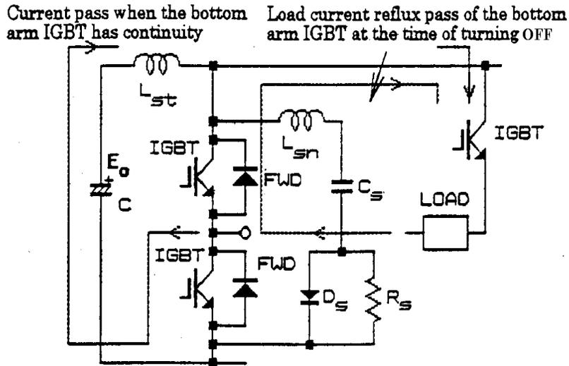
Figure 21. Turn-OFF Mode of bottom arm IGBT
