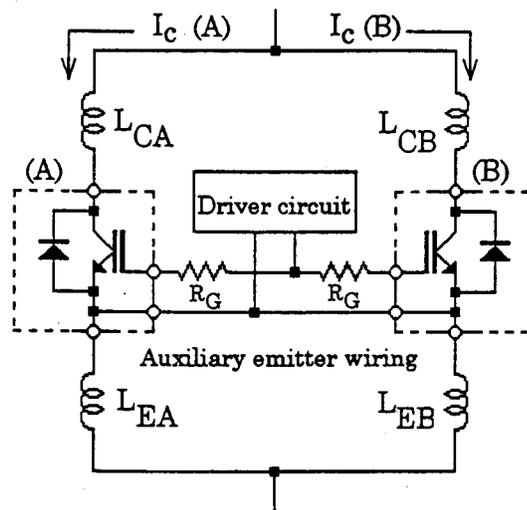
Figure 30. Wiring to equalize main wiring inductance values
