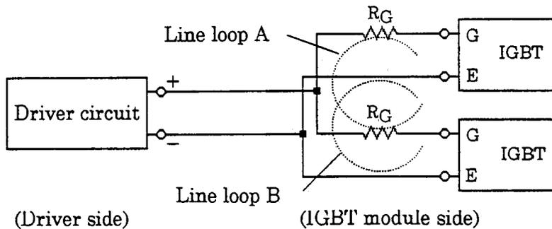
Figure 29. Parallel Connection between IGBT Modules and Driver Circuit
