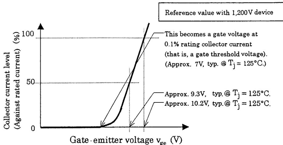
Figure 45. Gate Voltage - Collector Current Characteristics
