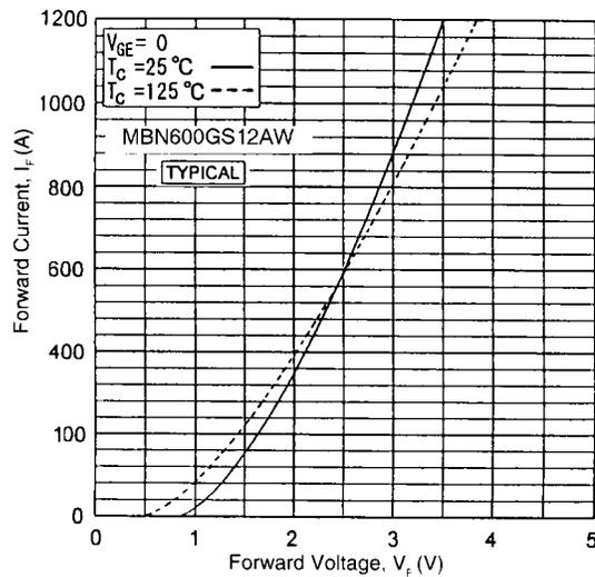
Figure 9. Forward Voltage Characteristics of a Free-Wheeling Diode
