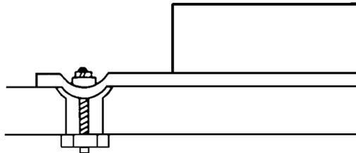
Figure 56. Example of Improper Heat Sink Mounting
